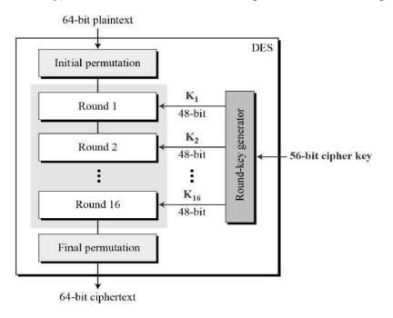
The initial and final permutations are straight Permutation boxes (P-boxes) that are inverses of each other. They have no cryptography significance in DES. The initial and final permutations are shown as follows
