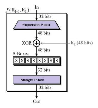
**Expansion Permutation Box** – Since right input is 32-bit and round key is a 48-bit, we first need to expand right input to 48 bits.
